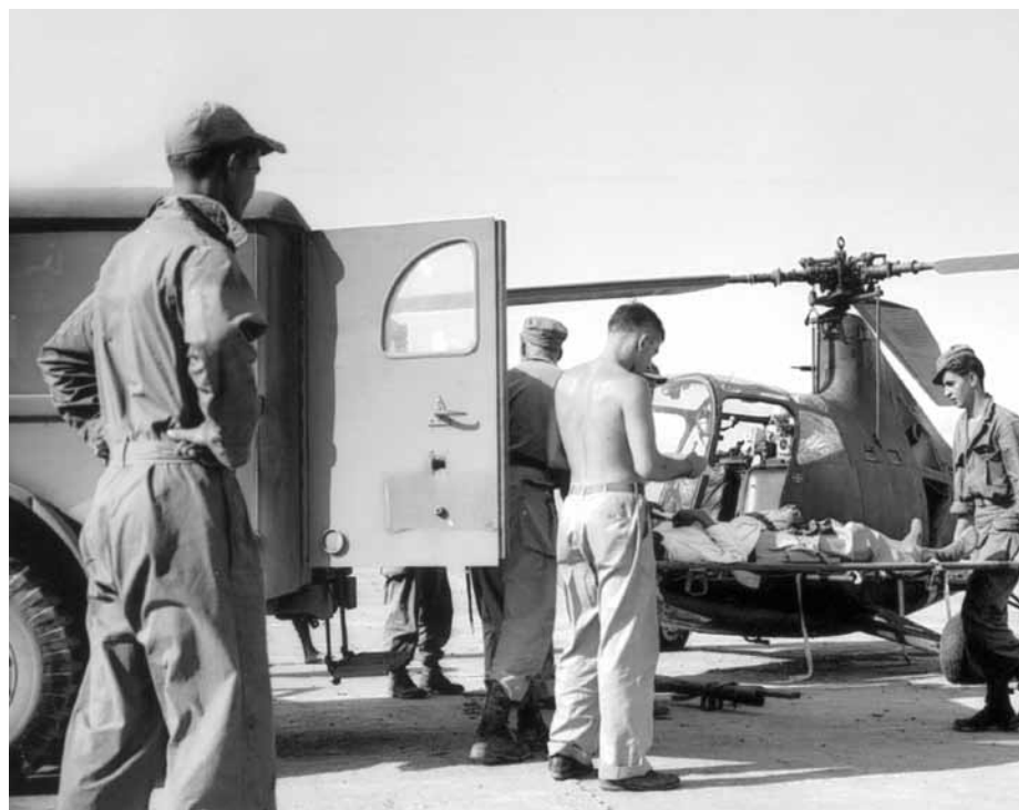
Some of the 6th ARUF pilots strapped the wounded to a Navy metal stretcher welded by two 1½ inch pipes to the helicopter.
