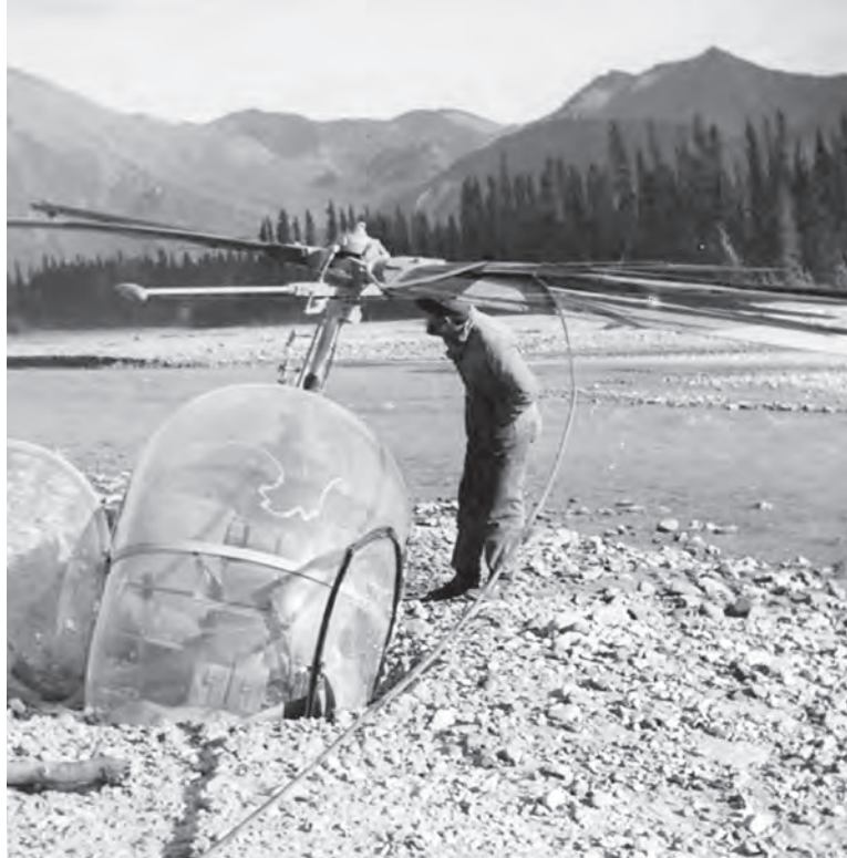
Ozzie inspecting wreckage of a submerged Bell 47 that had crashed in the Tok River in Alaska when the river was high.
